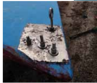
Since the broken shaft was no longer usable, a plate was bolted to either side of the rudder and lines attached to move the boat's rudder.
