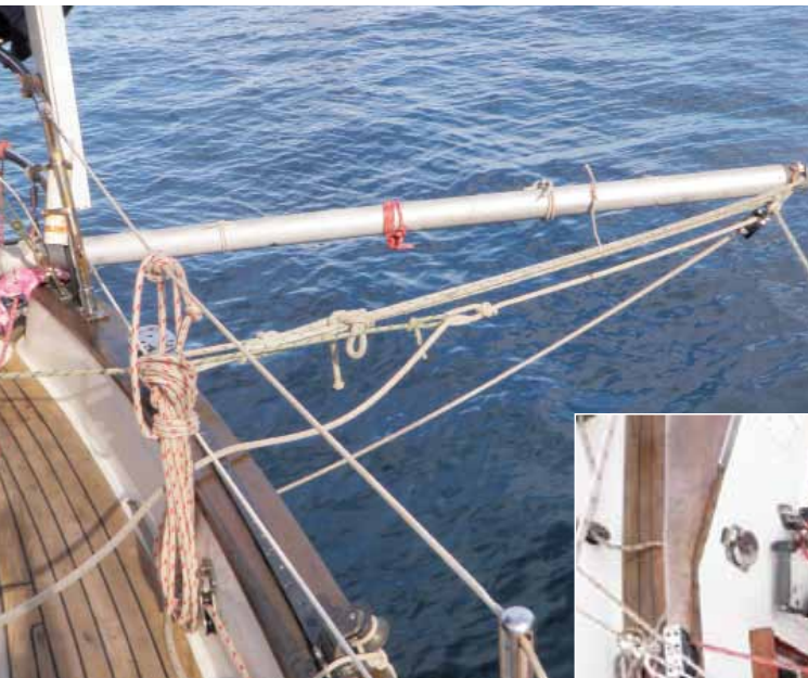
Left, a spinnaker pole, lines and blocks were pressed into service to control the steering lines. Below, the steering lines were led into the cockpit and onto a drum on Reality's wheel.
